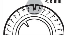
2. Repairs punctures up to 6 mm.
